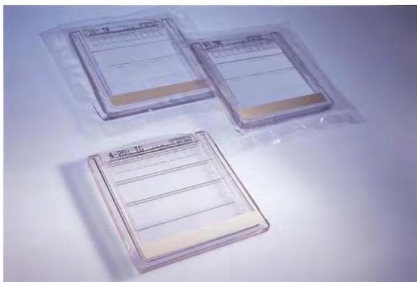
Tris-Glycin gels are suitable for general protein analysis. All gels have a stacking gel and do not contain SDS. By choosing the appropriate running and sample buffer (with or without SDS), native or denature conditions during the electrophoresis can be created. A wide spectrum enables the selection of the gel which complies to the applications.
